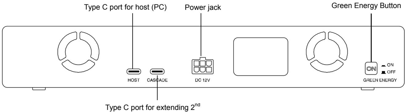
1. USB Type C Ports (Hub) - Allows connecting iPad, tablet or USB Type C mobile devices
