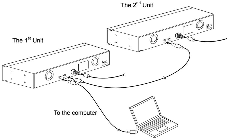
(2) Turn off the power switch of the 2<sup>nd</sup> unit.
